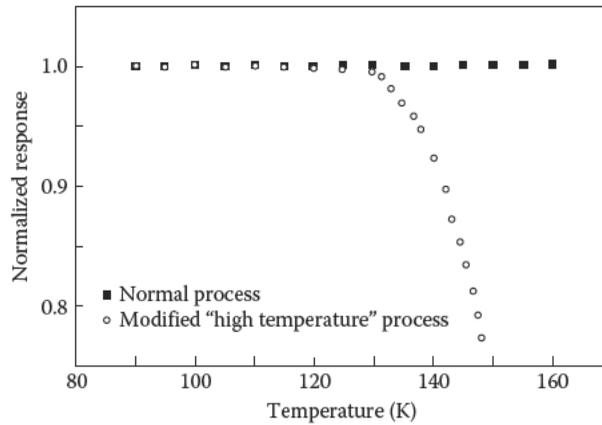
**Figure 13.26** Normalized response of InSb photodiodes in elevated temperature range. (From Wimmers, J. T., Davis, R. M., Niblack, C. A., and Smith, D. S., "Indium Antimonide Detector Technology at Cincinnati Electronics Corporation," *Proceedings of SPIE 930*, 125–38, 1988.)
